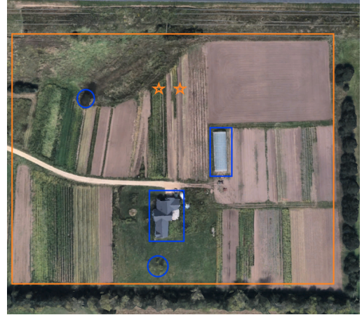
Fig. 4: Birds-eye view of the farm our solution is designed for. Within the perimeter (orange rectangle) of the farm, there are obstacles such as tall trees (blue circles), a house and a greenhouse (blue rectangles). Orange stars represent the placement of the UAV charging stations.
